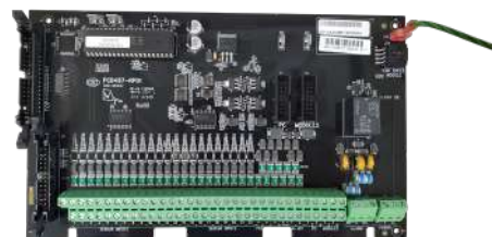
EXPERT Master Bottom Board (Number of Inputs Varies)
