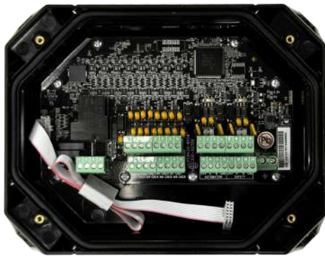
AA-811R-B AA128, Back Box & Board for AA-811R
