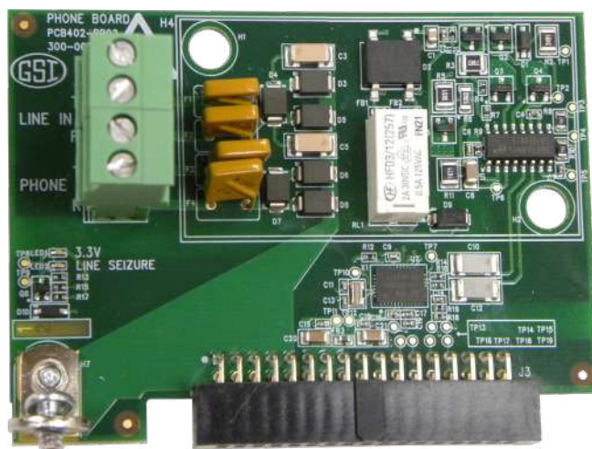
E330-0580 AA128, Phone Modem Card (Green Board)
