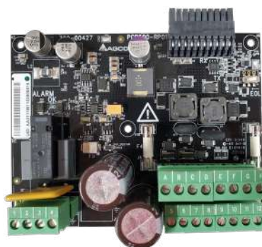
EDG2-003 EDGE 2 Main Controller Alarm and Communication Board
