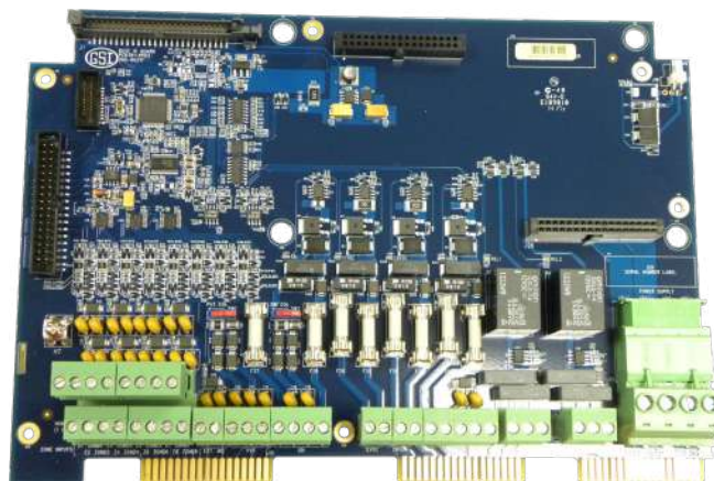
E330-0578 AA128, Master Bottom Board Only (Blue Board)
