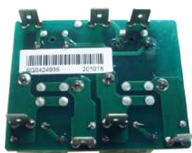
Old Style Relay Card Front & Back* E330-0490
