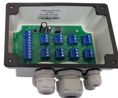
LOAD CELL JUNCTION BOX
